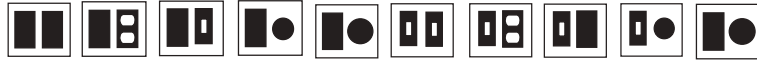
Double GFCI GFCI/Duplex GFCI/Switch GFCI/1-3/8" GFCI/1-5/8" Double Switch Switch/Duplex Switch/GFCI Switch/1-3/8" Switch/1-5/8"
